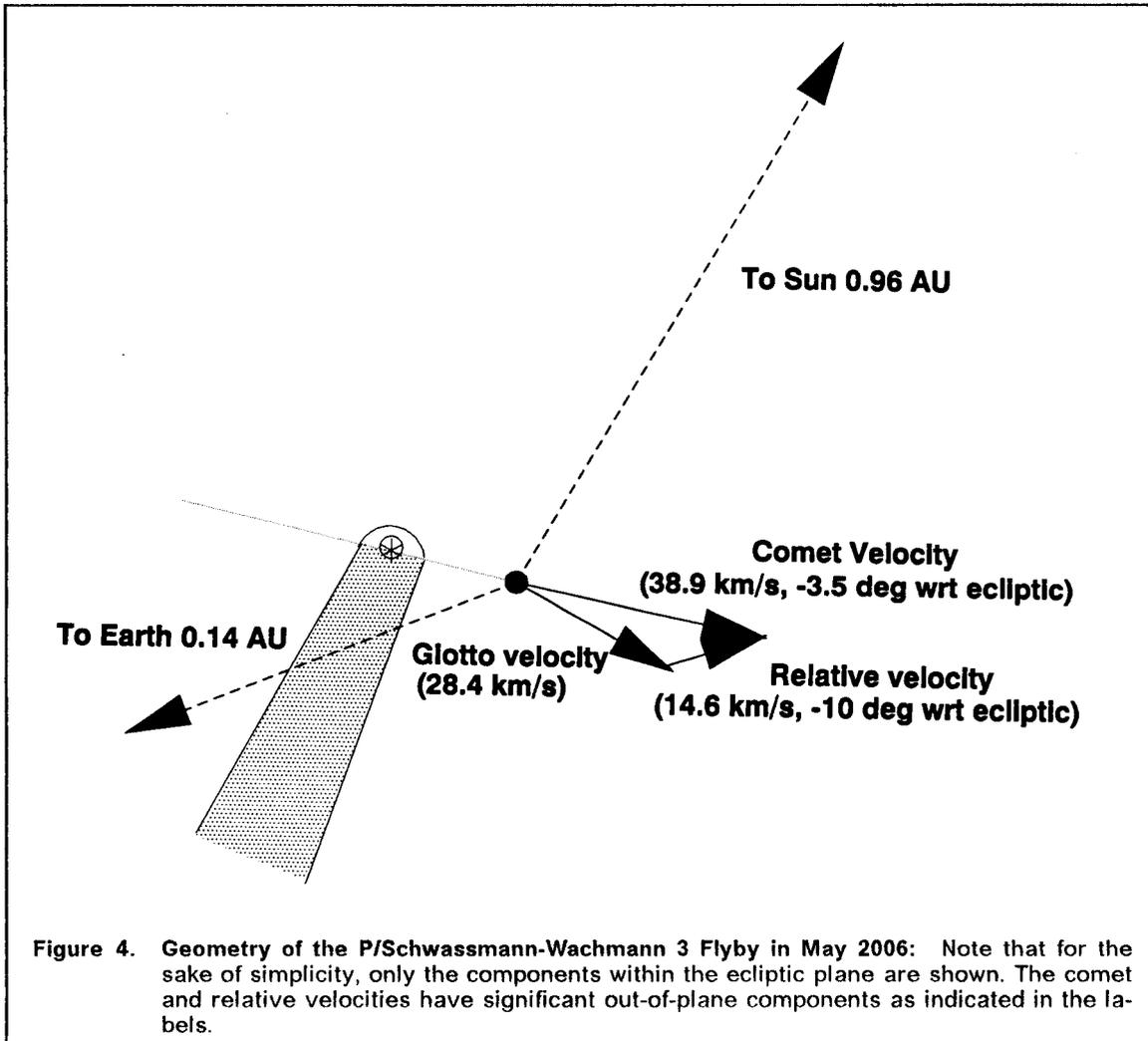
**Figure 4. Geometry of the P/Schwassmann-Wachmann 3 Flyby in May 2006:** Note that for the sake of simplicity, only the components within the ecliptic plane are shown. The comet and relative velocities have significant out-of-plane components as indicated in the labels.
